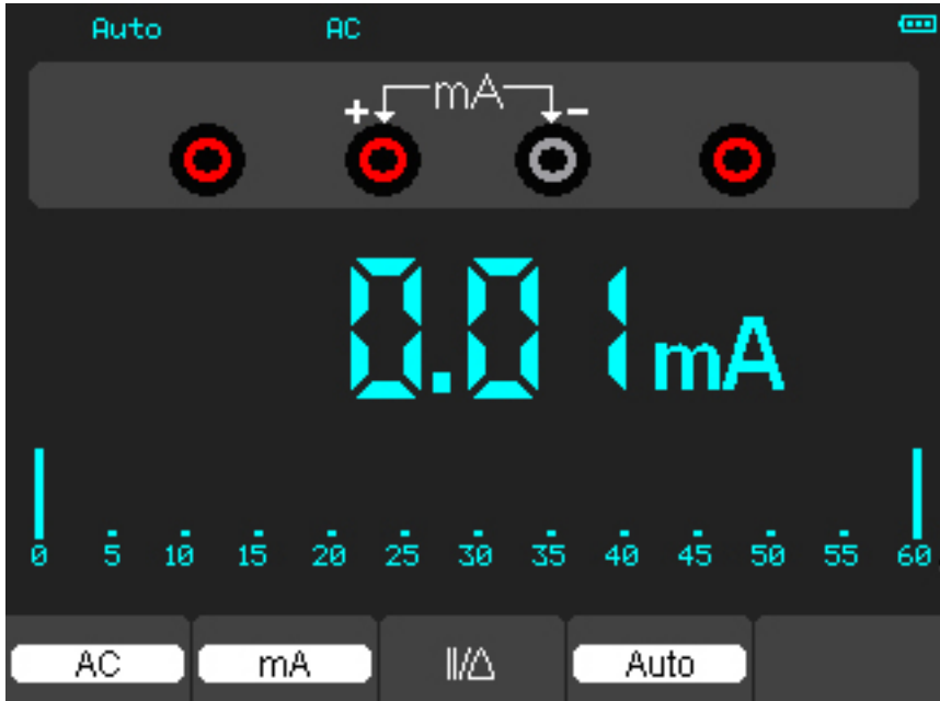
Figure 4-10 AC Current Measurement for 600 mA
