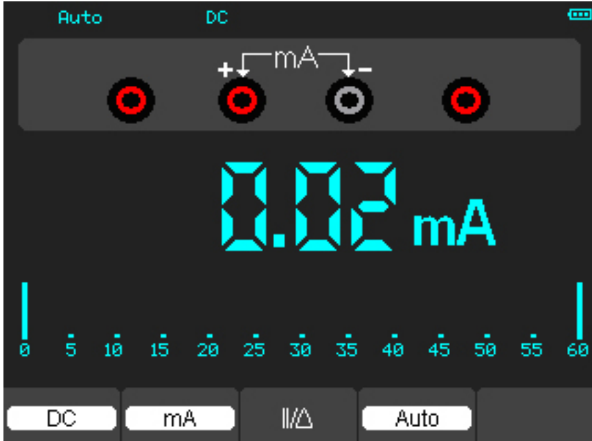
Figure 4-8 DC current Measurement for 600 mA
