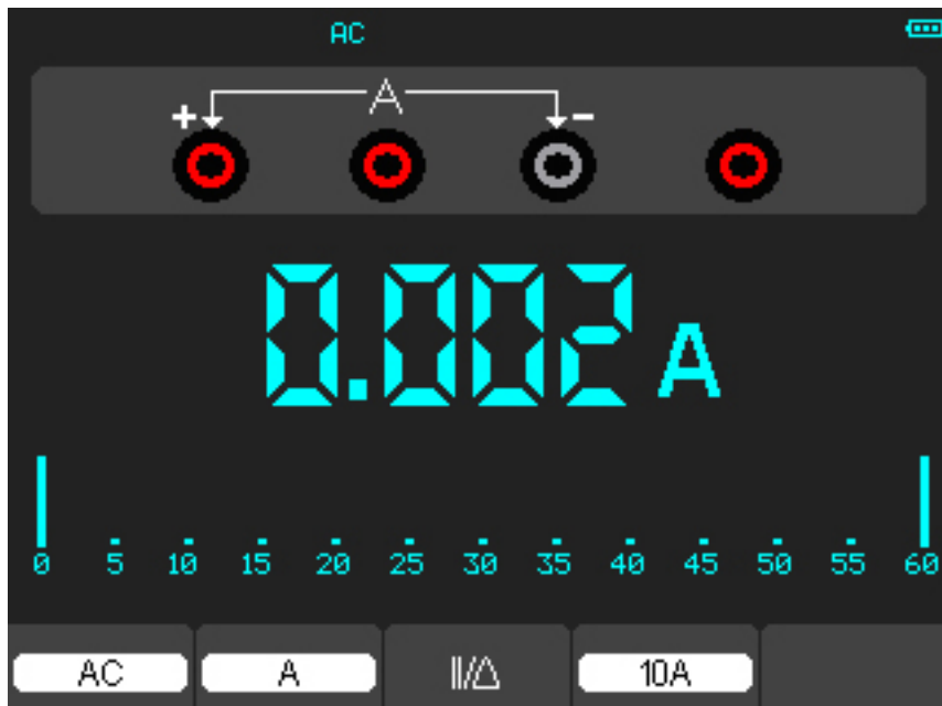
Figure 4-11 AC Current Measurement for 10A
