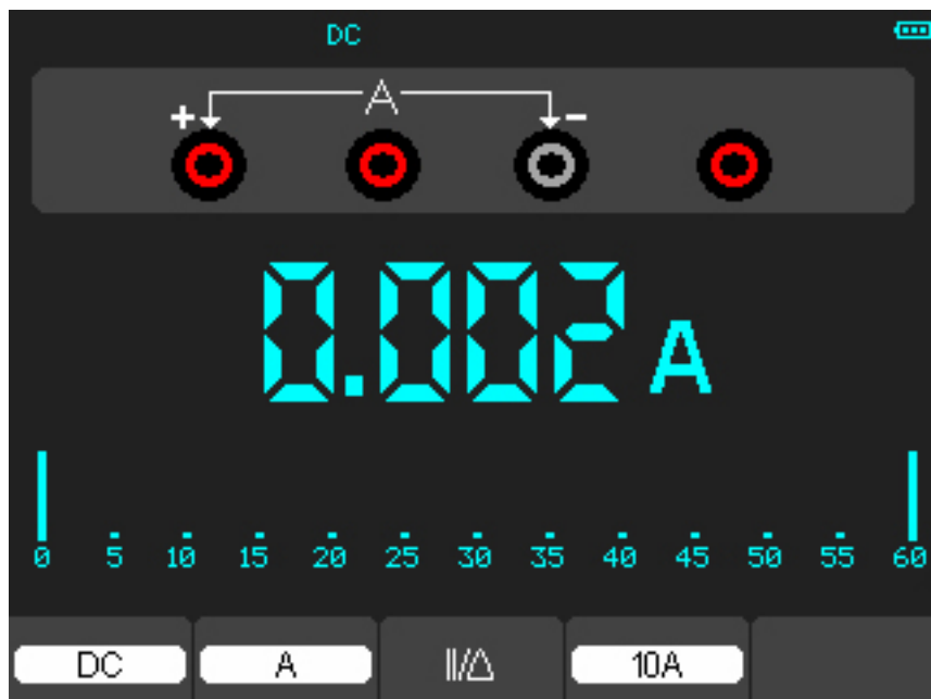
Figure 4-9 DC Current Measurement for 10A
